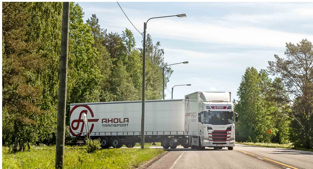
Proactive driving, in which the truck's rollout is used optimally, such as at intersections, saves both fuel and the environment.
